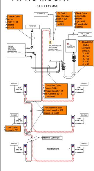
Cable lengths shown are standard based on number of landings ordered. Inclinator offers additional cable length options to meet non-standard installations. Please see order form for additional information on longer cable lengths
