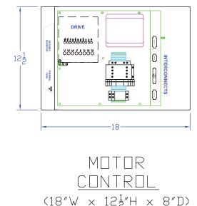
**NOTE**: The CPU/Controller and Motor Control is recommended to be mounted in the same location. However, up to 40' controller cables are available if needed.
