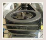
Three V-belts transmit power from motor to ACME screw.
